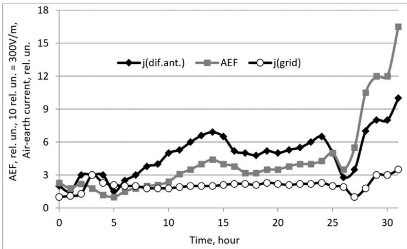
Figure 1.1.3: Synchronous recordings from the differential antenna  $j(\text{dif.ant.})$ , the field mill—AEF, and the gauge of “grid” type  $j(\text{grid})$ , obtained between 08h 00m 02/01/87 and 15h 00m 02/02/87. 31 hours of continuous recording under extremely adverse meteorological conditions: hours 2–4 fog; hours 10–15 strong wind; hour 26 snow showers; hours 29–31 strong wind, clear.
