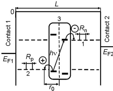
Fig.2.1. Diagram of energy levels in a sample with FPC and electrical contacts.
