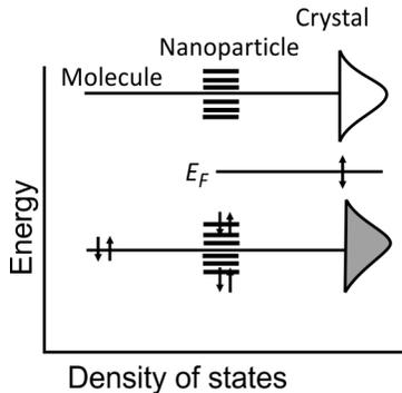
Fig.1.1. Electronic spectra of isolated molecules, nanoparticles, and crystalline semiconductor.
